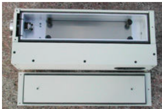
*Internal view of TL-105 Column Heater*
