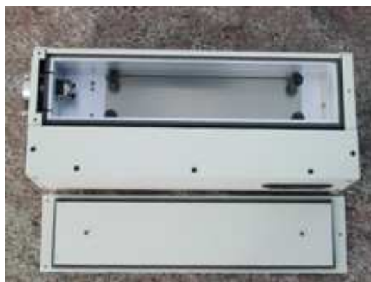
Internal view of TL-105 Column Heater
