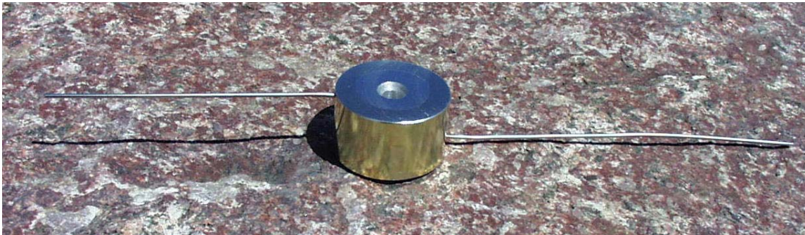
Figure 2: HX-101 Heat Exchanger
